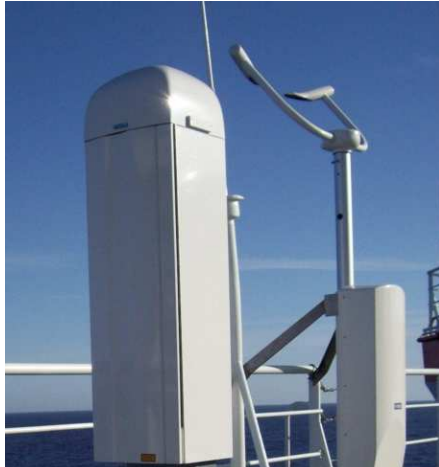
CL51 and Vaisala FS11 on research vessel Polarstern
